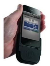
The iDynamo device should be attached to the appropriate adapter in order to be connected to either the iPhone or iPod Touch, or iPad. Once attached, the iDynamo can be connected to the iPhone or iPod Touch, or iPad.
